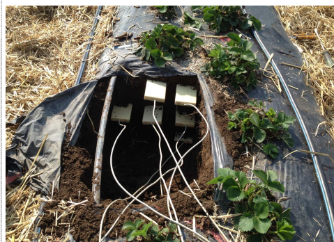
Figure 2. TDR probes inserted inside half of the raised bed
