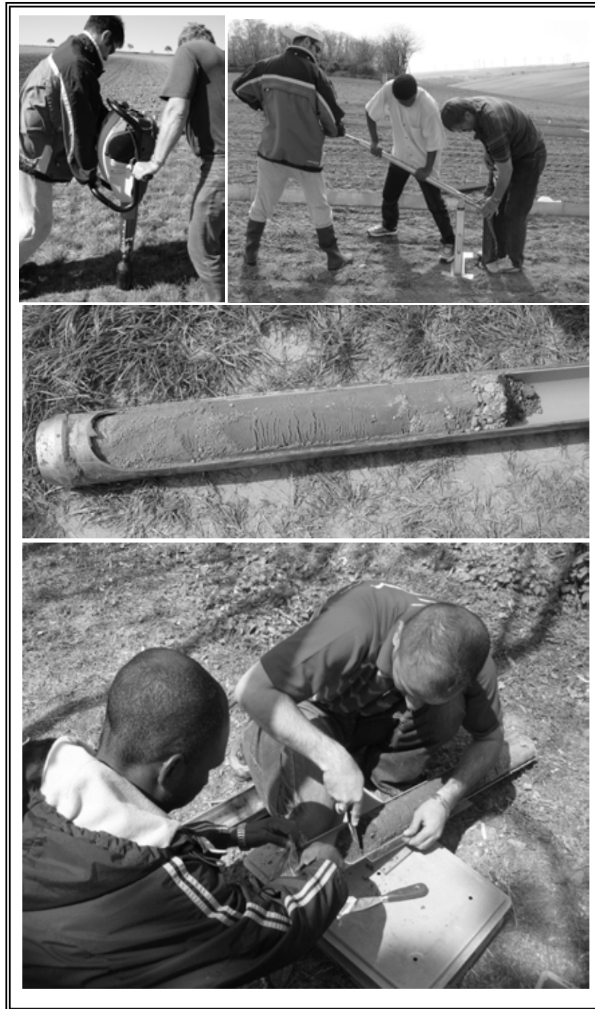
FIG. 8. Collection of soil samples by IAEA fellows and staff using a motorized soil column cylinder auger.
