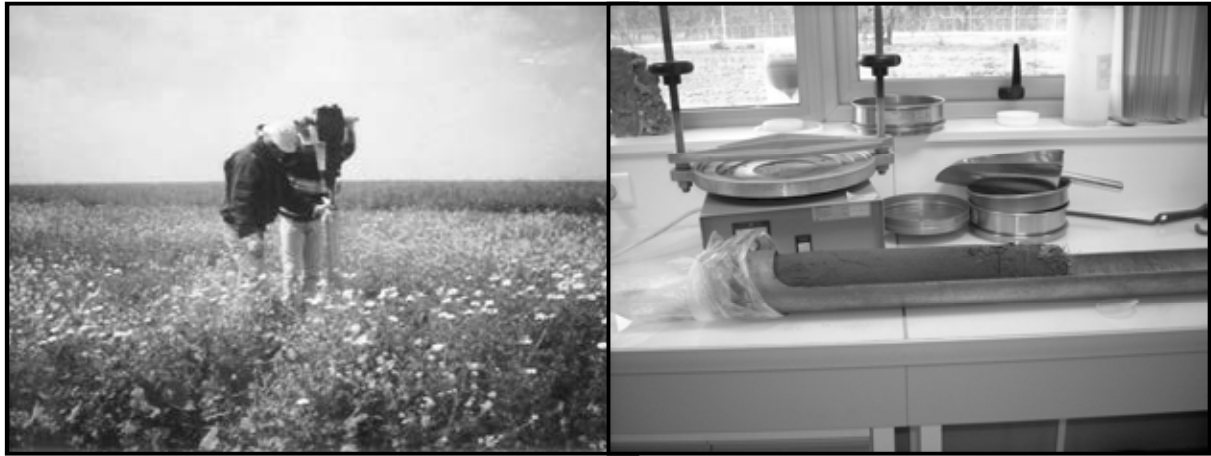
FIG. 3. Soil sample collection using a soil column cylinder auger and pre-treatment of a soil core at the CNESTEN laboratory.
