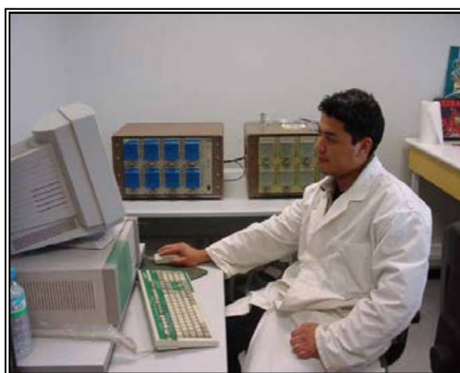
FIG. 9. Example of measurement of ^{210}\text{Pb} by HPGc “N-type” detector and alpha spectrometry (SSB detectors) via ^{210}\text{Po} at the CNESTEN laboratories.
