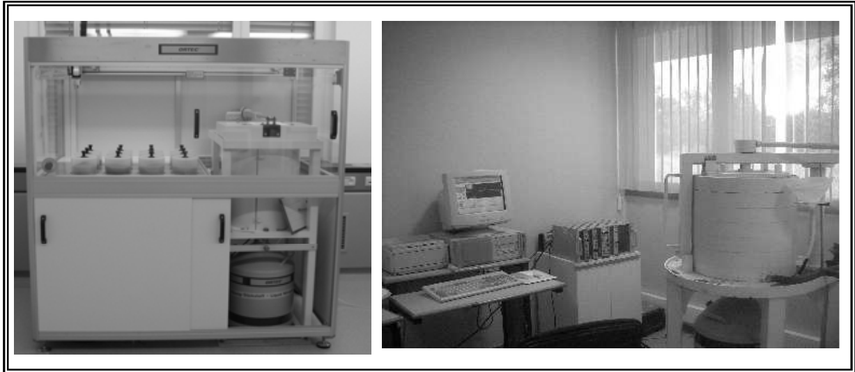
FIG. 12. Examples of HPGe detectors with shielding and electronic components at the IAEA Seibersdorf laboratory and at CNESTEN, Rabat, Morocco.
