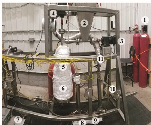
Fig. 1. Experimental set-up for black spruce pyrolysis: (1) nitrogen tank, (2) feeding hopper, (3) horizontal auger conveyor, (4) vertical auger conveyor, (5) heaters, (6) biochar container, (7) first condenser - glycol: water, (8) first bio-oil collector, (8) second bio-oil collector, (10) second condenser - chiller, and (11) non-condensable gases exhaust.
