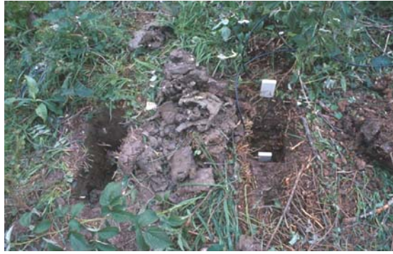
Figure 1. CS 615 sensor installation in heavy clay soil
