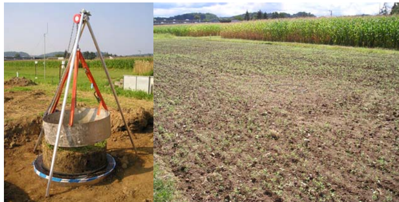
Figure 2. Integration of a Lysimeter into surrounding Vegetation in Wagna (Photo: Lanthaler).
