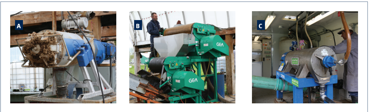
FIGURE 2. Examples of screw (A), roller (B) and centrifugal (C) separators
