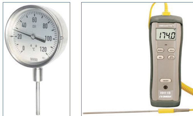
FIGURE 9. a) Dial or b) electronic thermometers for temperature measurements
